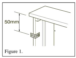
• Position the Hearth in place. Carefully move the Surround assembly into place. Ensure that the Surround is central to the Hearth. Mark the positions of the bracket holes on the wall. Move the assembly aside and drill suitable sized holes. Insert the wall plugs (L). Position the whole assembly into position and secure using two screws (M).
